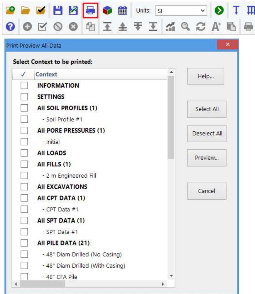
Using the 'Preview in Word...' option located within the secondary toolbar bypasses the above window and previews the data, results, or chart currently on the screen.
