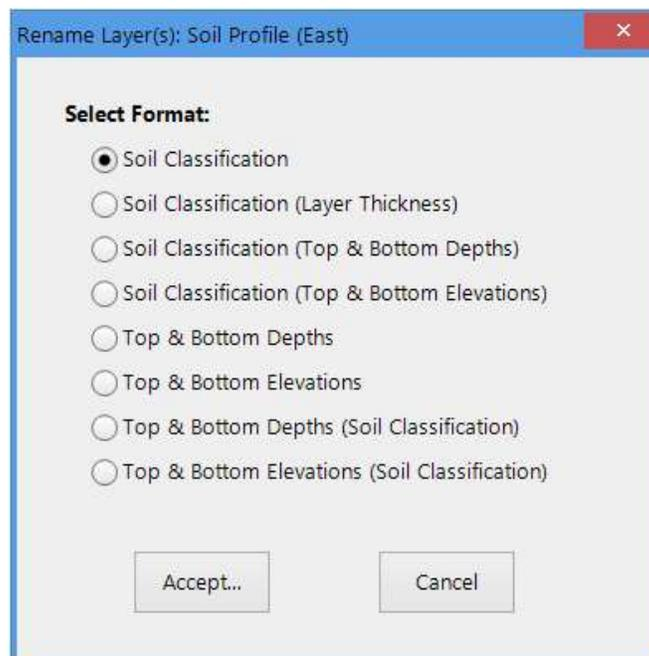
The name of individual soil layers does not affect the analysis itself. However, if named with consistency, this can make a project much easier to understand. Technically the name of a soil layer can be any alpha-numeric value up to 50 characters in length.
