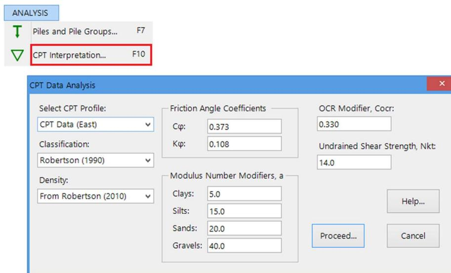
The main purpose of interpreting CPT data is to obtain a soil classification representing the dataset. UniPile 6.0 can analyze the data based on the three most popular soil classifications: Robertson (1986), Robertson (1990), and Eslami-Fellenius (1996). In addition to soil classification, the analysis will produce other useful
