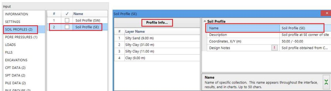
Within the 'Soil Profile' entry form, parameters related to an individual soil layer may be accessed by selecting it from the list. The entries relating to the soil profile in general may be accessed once again via the 'Profile Info...' button located at the top left of the form.
