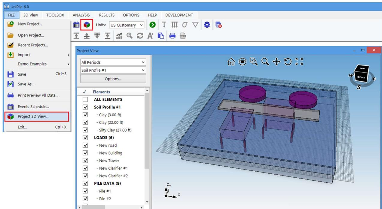
The list of the elements included in the project view includes soil layers, loads, fills, excavations, piles, and pile groups. Only one soil profile can be displayed at a time. Another soil profile, if specified, may be selected from the dropdown list.
