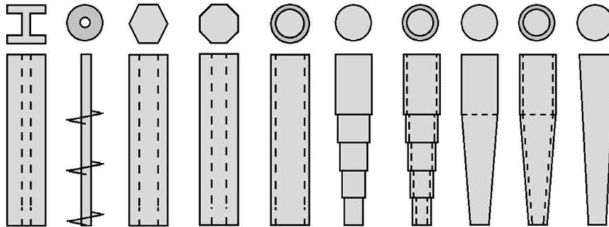
Pile type and geometry are identified by selecting from a list of available pile types. Pile types include but are not limited to Bored, CFA, Precast, Steel Pipe, Tapered Tube, H-Pile, Timber, and Helical. Steel pipe piles can be emptied or filled with concrete. Different toe geometry can be defined with a few keystrokes.
