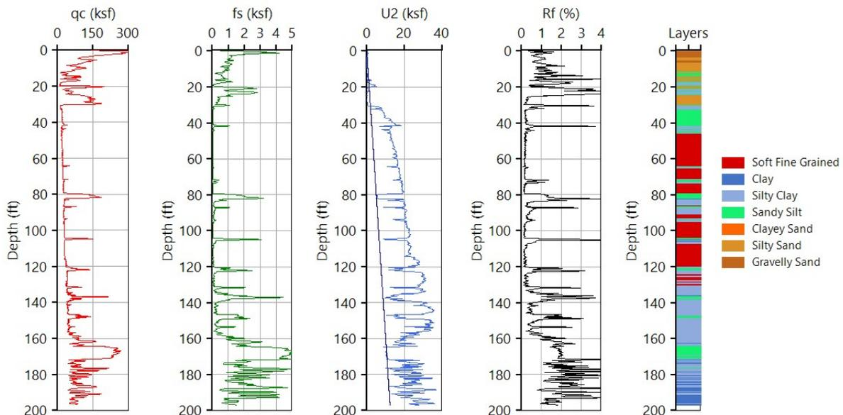
Results obtained from the interpretation of the CPT data may also be used to build a soil profile compatible with both UniSettle 5.0 and UniPile 6.0. This feature can be accessed via the 'Convert CPT Data to Soil Profile...' located within the main TOOLBOX menu.
