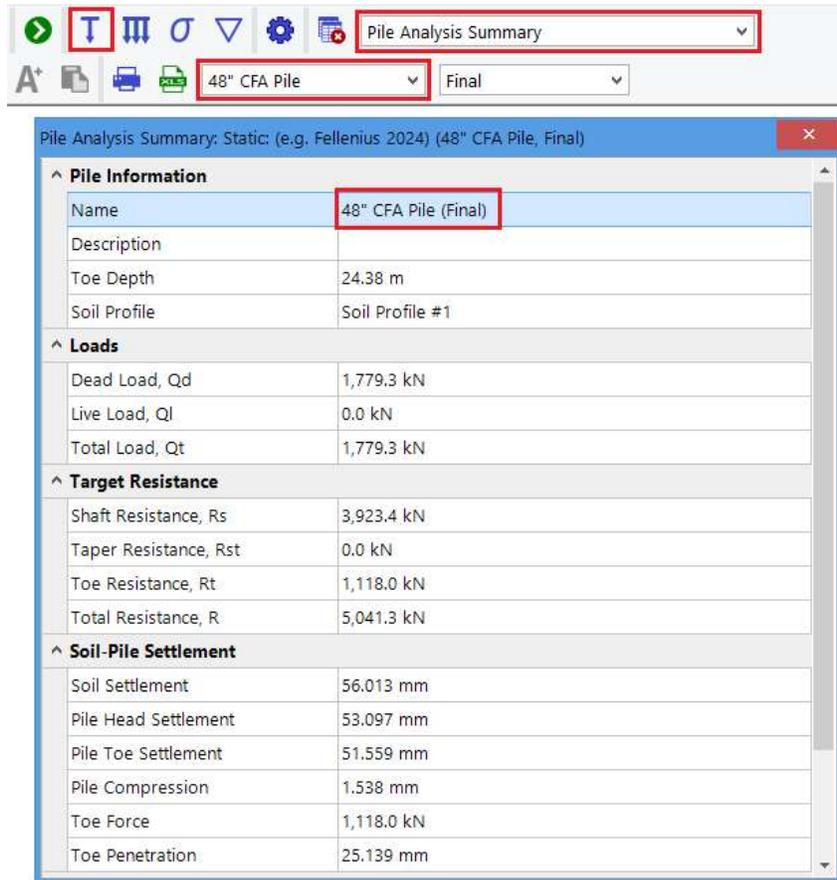
Depending on the extent of the analysis, UniPile 6.0 may produce up to 10 tables. Specific results are available inside the dropdown located within the primary toolbar.
