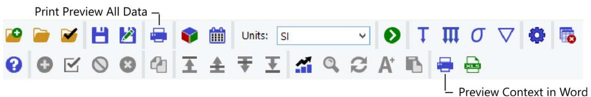
The 'Print Preview All Data...' opens a window allowing the selection of one or multiple sets of input data. Depending on the size of the project, previewing all data may produce hundreds of pages and may take a few minutes. This is particularly the case when CPT datasets are included.
