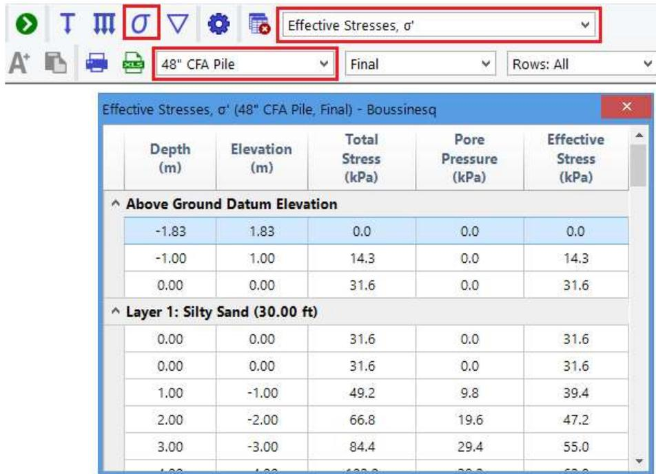
Effective Stresses,  $\sigma$  (48" CFA Pile, Final) - Boussinesq
